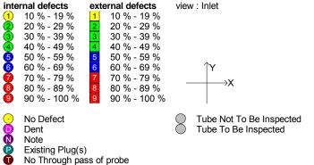
: Cooler A subject 1 from 1 page(s) client Client a Msite b site order-no. : K-xx0-16 K.-No. : 17.10.2016 Date Material : A789 Duplex Tube length : 9600 mm : 25.40 mm Ø External Ø Internal : 22.10 mm Wall thickness: 1.65 mm
