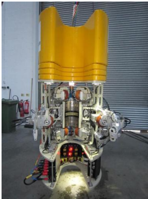
Figure 14: The MEC-HUG™ tool for the inspection of flexible riser for top-side deployment.
