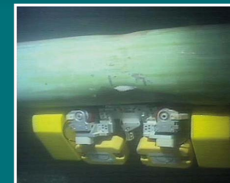
In these pictures: External underwater inspection of subsea pipelines and assets with the smart, multi-function MEC-Combi inspection tools.
