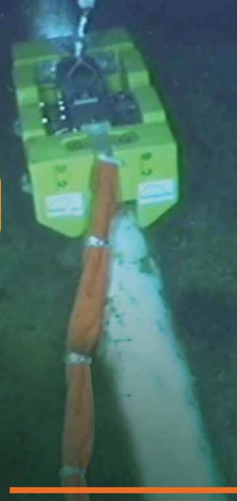
The inspection results show excellent signal to noise ratio which confirmed the high detection capabilities of the MEC-Combi Crawler with limited preparation of the pipes.
