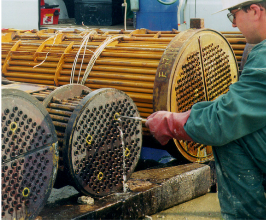
Inspector manipulating the IRIS probe. Tubes are plug at the other end and flooded with the turbine.
