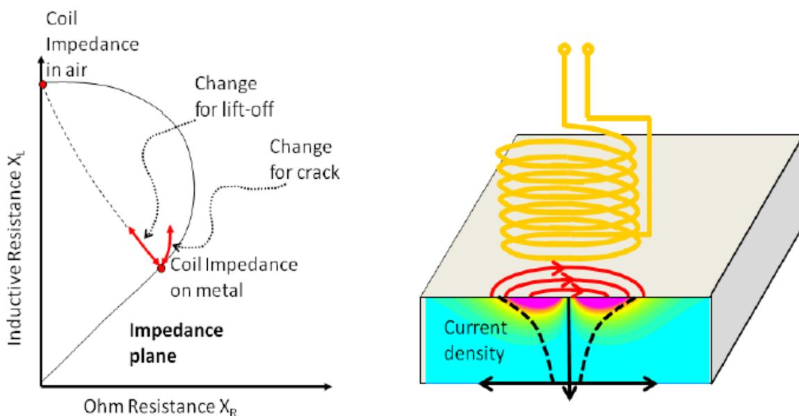
Figure 2: Left – The impedance plane shows the signal in two dimensions.
