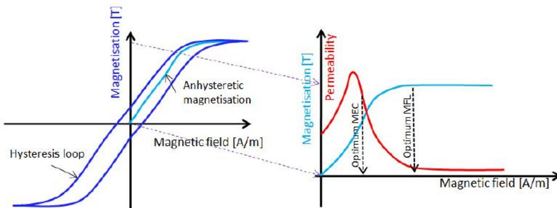
Figure 4: Change of permeability with magnetisation level
