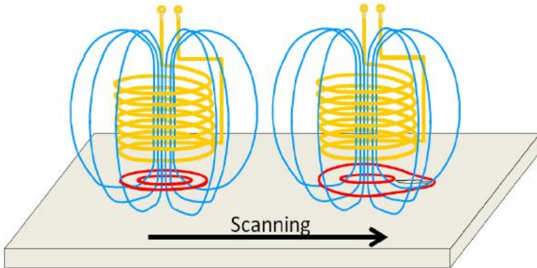
Figure 1: The concept of eddy current testing
